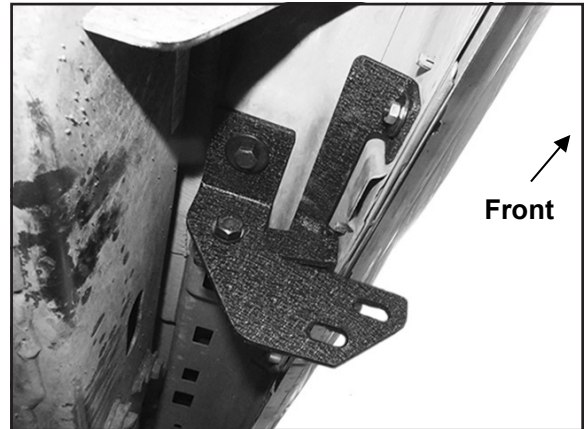
(Figure 5) Driver/left front Brackets installed.
